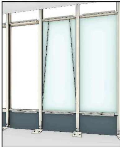
Install the interior vertical glazing beads
