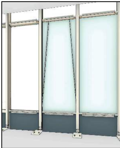
Install the interior vertical glazing beads
