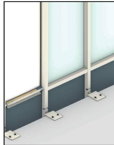
Install the interior cover cap
