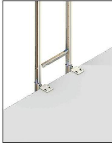
Bring the transom into a horizontal position, rotate and click it in the mullion cutouts
